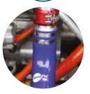
Simple and secure solution for quick release radiators and intercoolers, AeroFlo™ eliminates complex tube bending issues.
